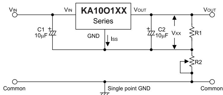
Circuit for increasing output voltage
